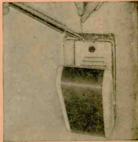
Photo 6—The new latch bolts are soldered in.
